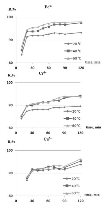
Fig. 4. Influence of temperature and time on sorption of heavy metal ions (pH  $= 7.0 {\pm} 0.1$
