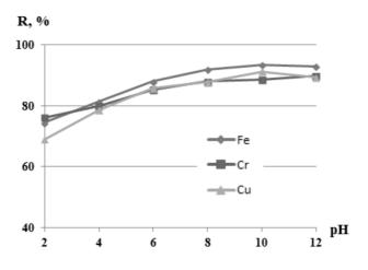
Fig. 3. Effect of pH on sorption of heavy-metal ions
