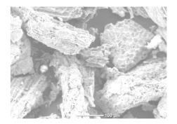
Fig. 1. Activated carbon sorbent received as a result pyrolysis of silt rainfall
